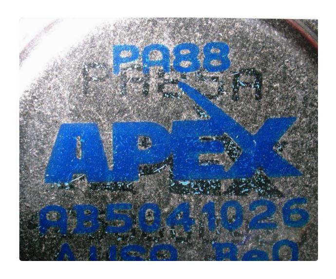
Parts passed test (re-marking substance was resistance to solvent). However, closer inspection revealed ghost markings.
